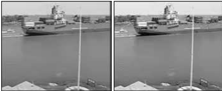
Fig. 6. 16th frame of “Container” coded with MP (left) and 8x8 DCT (right)
