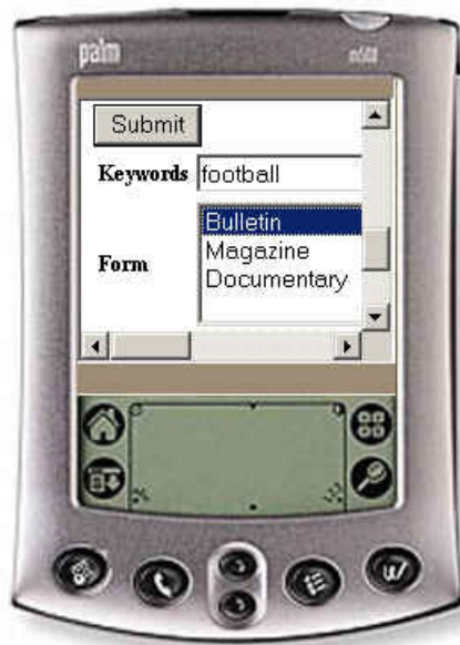
Figure 6.8: Results Page of the UMA Demonstrator: user fills the form situated beneath the list to search for specific content
