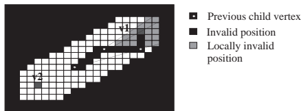
Figure 7. Dynamically reduced set of positions for child vertices along a level 2 parent edge, 3 previously transmitted child vertices, geometrical rule (8).
