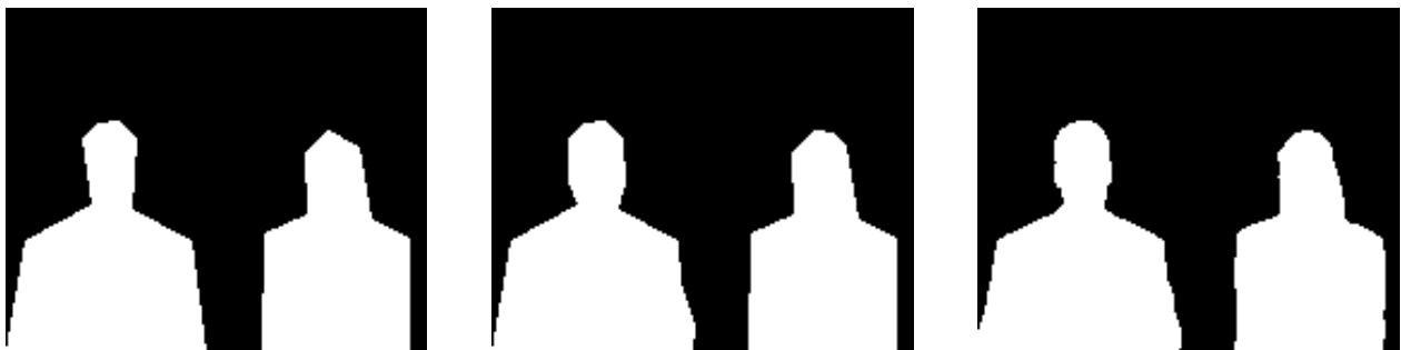
Figure 8. Progressive decoding of sequence 'News', frame 0. From left to right: coarse approximation (error 2, 341 bits), intermediate approximation (error 1, 416 bits), lossless representation (1087 bits).
