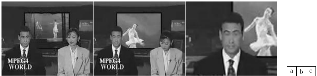
Figure 19: Reconstructed frames of News at 48 kbit/sec. (a) Frame #1 (b) Frame #300 (c) Zoom on face area frame #300
