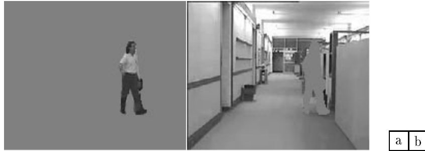
Figure 21: Reconstructed frames of Hall monitor compressed at 48 kbit/sec with the object-oriented configuration. (a) Frame #300 foreground object only, (b) Frame #300 background object only
