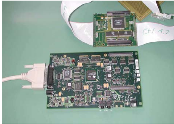
Figure 4.6: The TMS320C6711 DSP Starter Kit (bottom) with a mezzanine card containing a first implementation of the L1 Buffer (top) used for first tests. Asynchronous memory has been used for the L1 Buffer.
