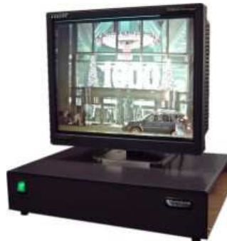
Figure 5.1: HDR display prototype. This Figure was taken from (Seetzen et al. 2004).
