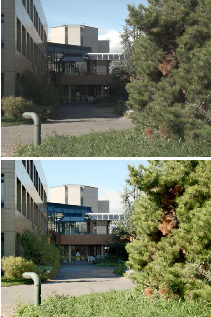
Figure 3.25: Results of the Retinex-based adaptive filter method. Top: Gamma-encoded image. Bottom: Image treated with our method. This image is from our database.
