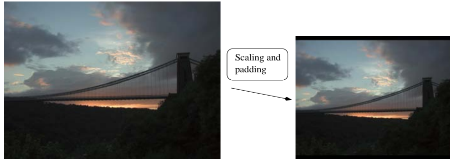
Figure C.2: Scaling and padding. The input image is scaled to the display resolution. Zero-padding is used if the aspect ratio of the source differs from that of the display.
