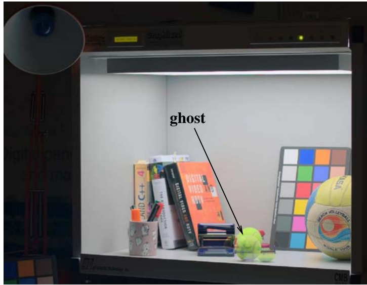
Figure B.1: Example of ghost caused by a moving object in an HDR scene captured by a multiple exposure technique.
