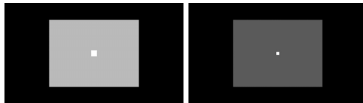
Figure 5.12: Generated images for measurements. Left: Background: 50% of \Psi_{max} , Specular highlight size: 1.1 degree. Right: Background: 10% of \Psi_{max} , Specular highlight size: 0.55 degree.
