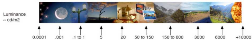
Figure 1.1: Maximum luminance values for various scenes. This Figure was taken from (Johnson 2005).
