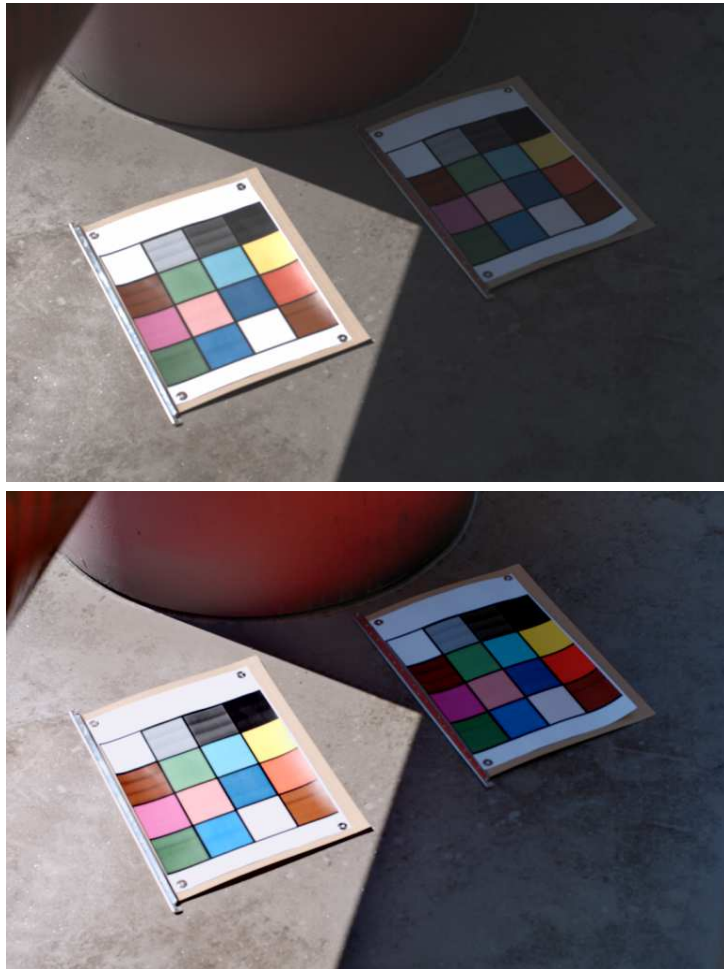
Figure 3.26: Results of the Retinex-based adaptive filter method. Top: Gamma-encoded image. Bottom: Image treated with our method. This image is from our database.
