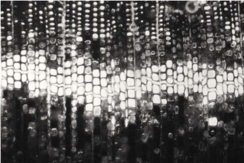
Figure 7-18 Spruce in Mode I, RL orientation fracture test, the developed crack in earlywood has more intercellular form than intracellular one (Job L. Navi P. 1996)
