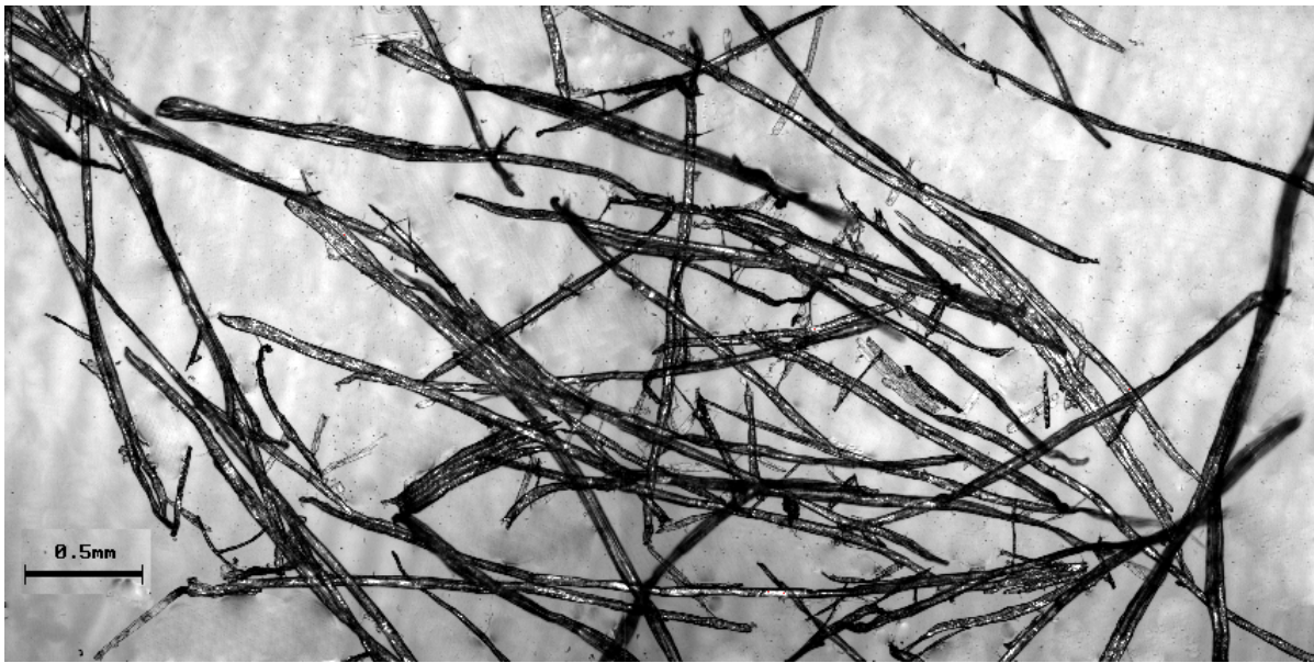
Figure 3-1 Macerated spruce fibers in an acidic based solution
