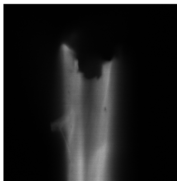
Figure 4-16 Failure point in a latewood fiber
