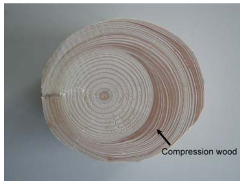
Figure 2-12 Compression wood is recognized by the change of color in transversal cut of a spruce trunk
