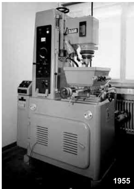
Figure 1.6: 50 years of evolution in EDM machines: Eleroda D1 (1955) and Robofil 2050 TW (2005) from Charmilles (images © Charmilles Technologies [1]).
