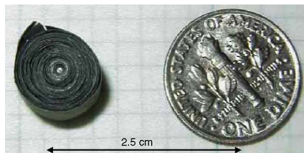
Fig. 10. Microchannel catalyst for autothermal reforming of hydrocarbon fuels [81].
