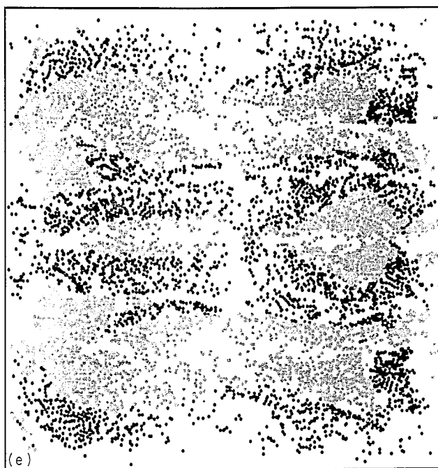
Fig. 12. Particle configuration at reactor outlet for a single static mixer with various crossing angles: (a) 10°, (b) 30°, (c) 60°, (d) 90°, (e) 120°.
