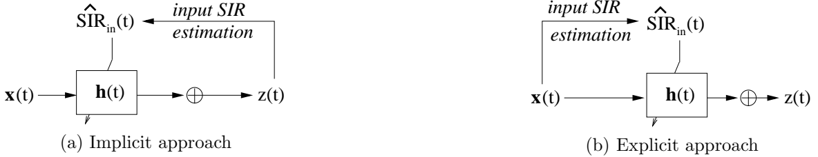
Figure 2: Implicit and explicit adaptation control. \mathbf{x}(t) = [x_1(t) \cdots x_M(t)]^T are the signals captured by the M microphones, and \mathbf{h}(t) = [\mathbf{h}_1(t) \cdots \mathbf{h}_M(t)]^T are their associated filters.
