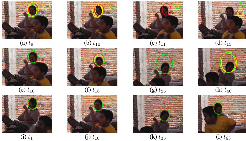
Figure 8: Head tracking 1 : first row : shape-based tracker M1. Second row : shape-based tracker M2. Third row : shape-based tracker M3. In red, mean state; in green, mode state; in yellow, likely particles.
