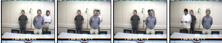
Figure 9: Tracking results for RealSeq2 . PS ( 1 \rightarrow 2 \rightarrow 3 ) fails to recover from occlusion (frames 2,20,40,120 shown) success and recovery rate: 8%. Particle (u, v) positions are superimposed on the image. Brighter pixels indicate higher likelihoods (139 frames at 360x288). On the contrary, DPS has higher success and recovery rates: 60% and 88% respectively.
