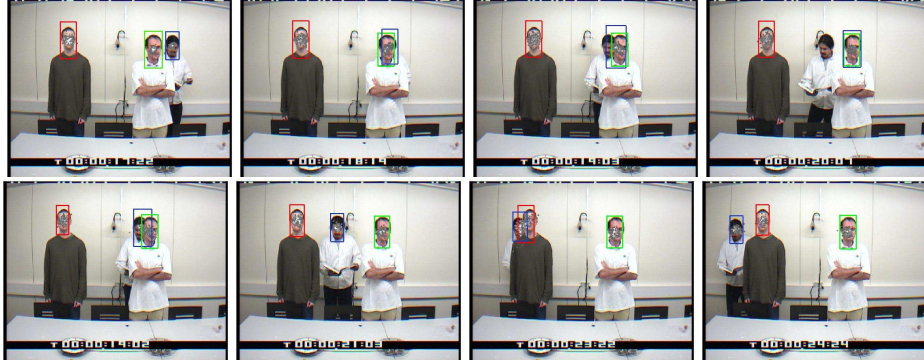
Figure 7: Tracking results for RealSeq1 . Top: PS method fails to recover from occlusion (frames 10,32,41,70 shown). Bottom: DPS method recovers from occlusion (frames 40,91,160,197 shown). (191 frames at 360x288).
