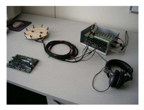
Figure 6: Small microphone arrays, and its realtime hardware, typically used in the IDIAP smart meeting room to perform acoustic source localization.
