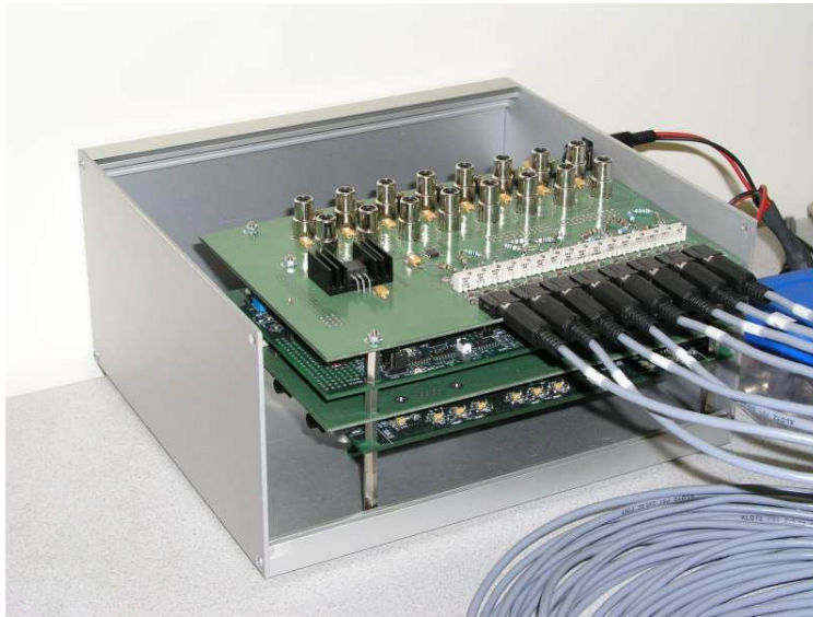
Figure 4: Small Microphone Array Hardware
