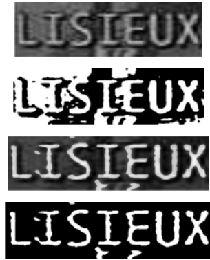
Figure 8 (a) original image, (b) binarization result of the image, (c) enhanced image using proposed method, (d) binarization result of the enhanced image
