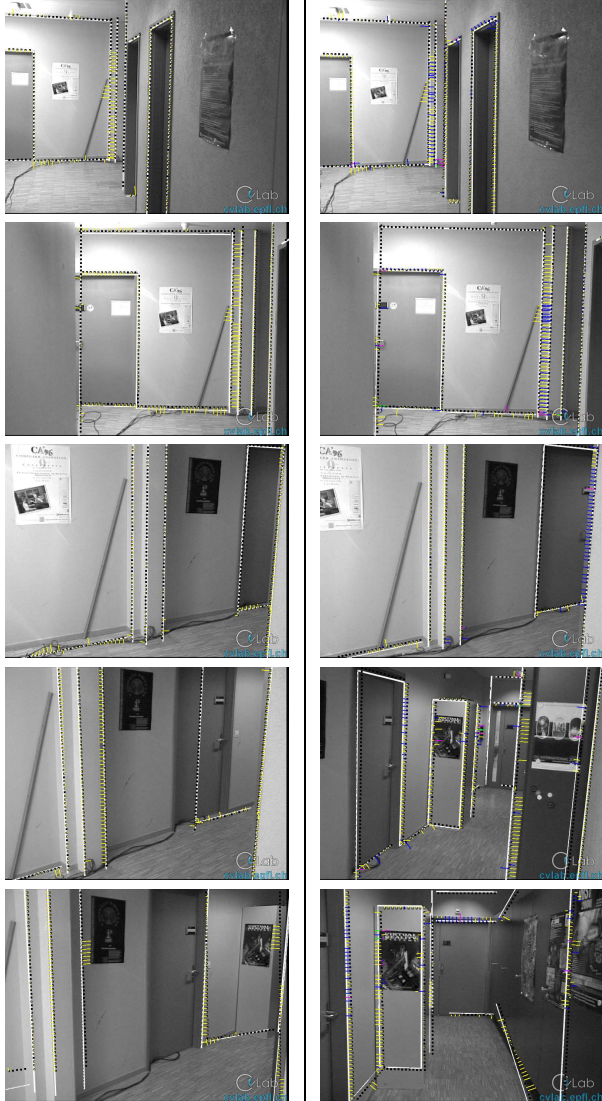
Figure 3. CORRIDOR SEQUENCE, USING EDGE INFORMATION ONLY. First column: When considering only one hypothesis per edge point and no interest points, the right side of the door is attracted by the right wall (pictures 4 and 5) and the tracking eventually fails. Second column: Considering multiple hypotheses as we propose makes the tracking more robust. Nevertheless the reprojected 3D model sometimes jitters. Integrating the texture information suppresses this problem.
