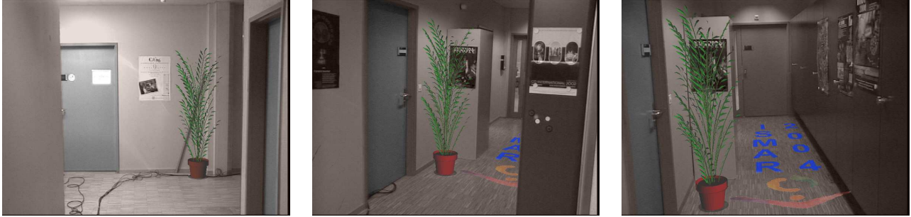
Figure 9. AUGMENTED VERSION OF THE CORRIDOR SEQUENCE. The corresponding video sequence can be found at the following address: http://cvlab.epfl.ch/research/augm/augmented.html . Thankful to the edge information, occlusions between the real scene and the virtual objects are precisely handled. When watching the sequence, the reader can see that the virtual objects do not jitter or drift.
