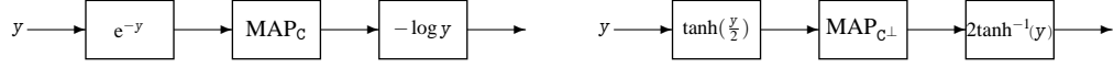
Figure 2.10: Two equivalent implementations of a decoder with L -values at input/output. The MAP decoder uses ratios as inputs/outputs, e.g., it is a simple product for the case of a repetition code. Left: Implementation based on the actual code and its MAP decoding. Right: Implementation in the dual domain.
