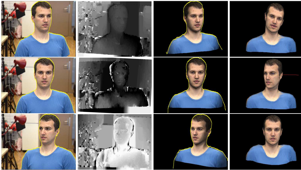
Figure 6. Reconstruction from an uncalibrated video sequence. Left column: 3 of 6 images from a short video sequence with overlaid silhouettes on head, neck and shoulders. Second column: Disparity maps extracted from rectified consecutive image pairs using max flow-based stereo, after automated registration. Third column: Textured reconstructed model with triangular metaballs where overlaid silhouettes show correct fitting to silhouettes. Forth column: Animated reconstructed model.
