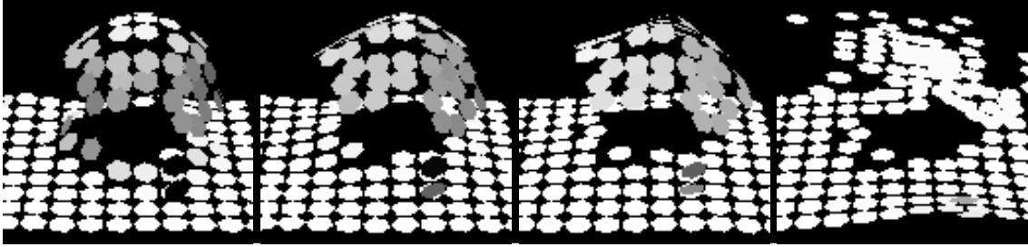
Figure 7: Rearranging the particles of the second row of Figure 5 by minimizing the deformation energy alone. The optimization progresses from left to right. All particles, but only a few outliers, end up lying on one of two separate planes.
