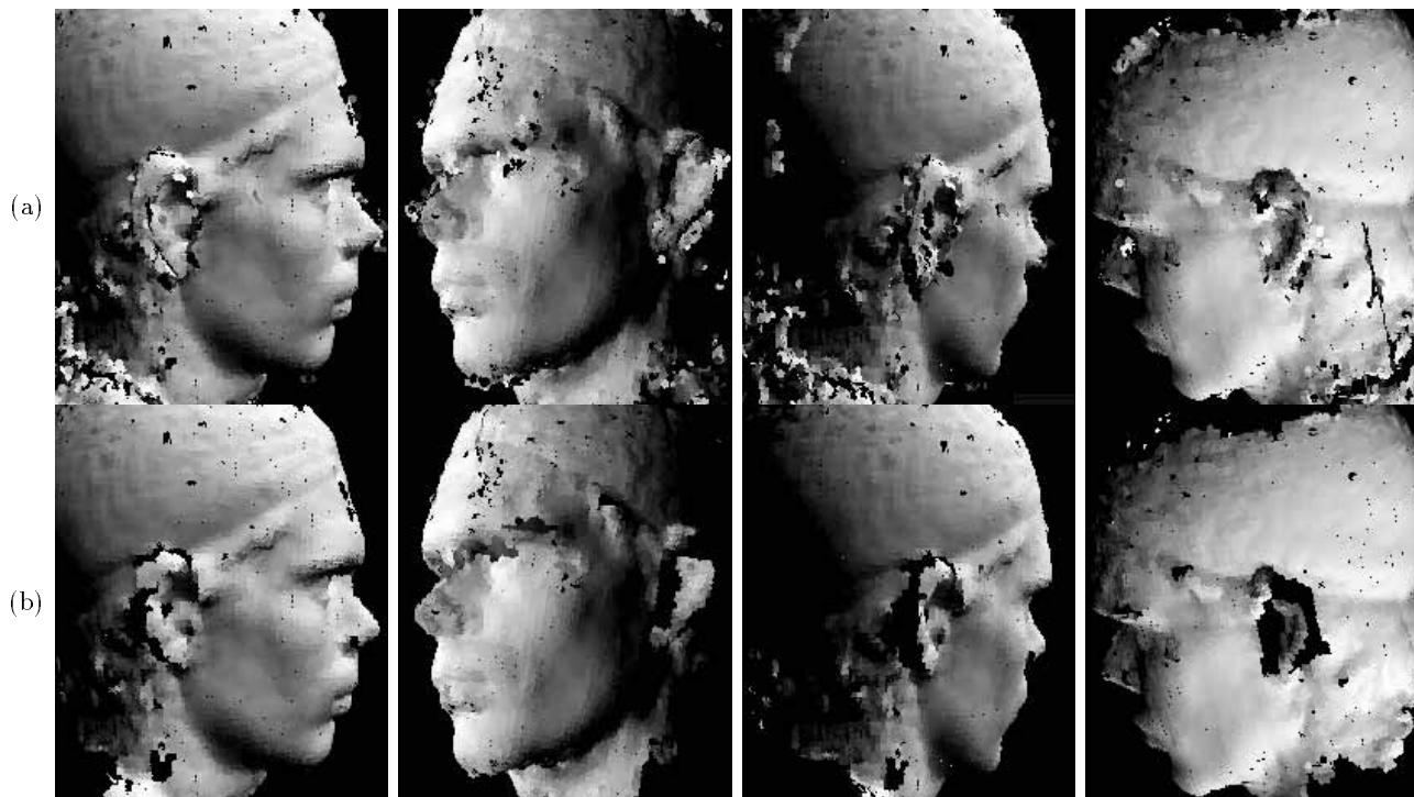
Figure 9: Modeling the head. Row (a): Four shaded views of the particles instantiated by fitting local surfaces to the 3-D points derived by correlating the images of Figure 8. Row (b): Similar views of the subset of particles that belong to the same global surface. Erroneous ones on the side of the nose and the back of the head have been eliminated.
