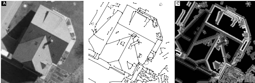
Figure 3 (A) a cut-out 350 \times 350 from the dataset in Fig.1, (B) The resulting attributed graph with all its contours and vertices, (C) the flanking regions with their corresponding median luminance attributes. The background is black.
