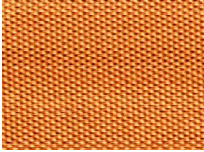
Figure 3.1: The clean Ag(111) surface observed with STM at a base temperature of T = 50 K with a tunneling voltage of V_T = -20 mV and a setpoint current I_T = 1 nA. The size of the image is approximately 9.5 \times 7 nm 2 .
