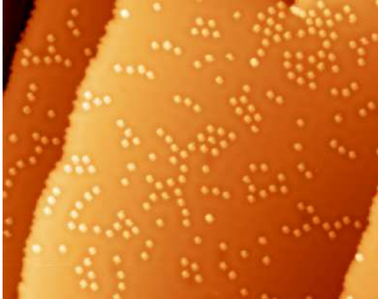
Figure 3.6: STM constant-current image of the Ag(111) surface covered by approximately 0.2% of a ML of Ce obtained at a temperature of 3.9 K (image-size 100 \times 80 \text{ nm}^2 , V_T = -100 \text{ mV} , I_T = 20 \text{ pA} ). The Ce adatoms have a preferred next-neighbor distance of 3.2 nm.
