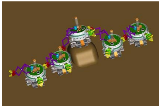
Figure 9. Graphic visualization of how lateral semi-flexible connections are going to be used to keep relative mobility between s-bots while they are in a swarm-bot configuration. This flexible structure can help for instance to pass local small obstacles.
