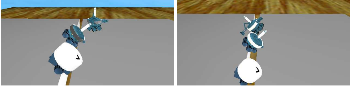
Figure 21. From left to right: The 3 s-bot models while traversing a gap of 40 mm and 60 mm, respectively.
