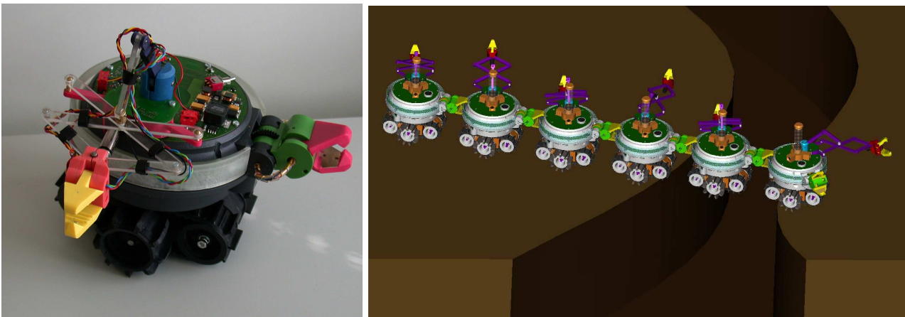
Figure 5: Left: The prototype of the s-bot robot with the strong beak gripper and the flexible arm. Right: Several s-bot robots can attach to build a swarm-bot capable of passing obstacles one single s-bot cannot deal with.
