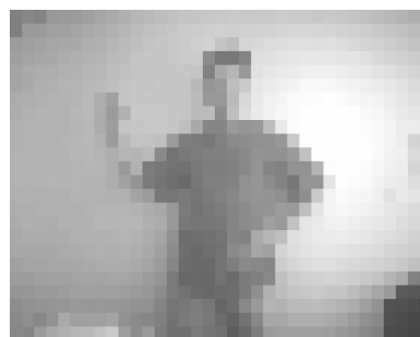
Fig.8 2D sub-sampled image (35x24 pixels) from OV7645FB camera. The camera is wired to PEvoPic via a flex connector supporting. The microcontroller is programmed to grab the frame, store the 840 pixels in its data memory before sending them upon request to a desktop computer.
