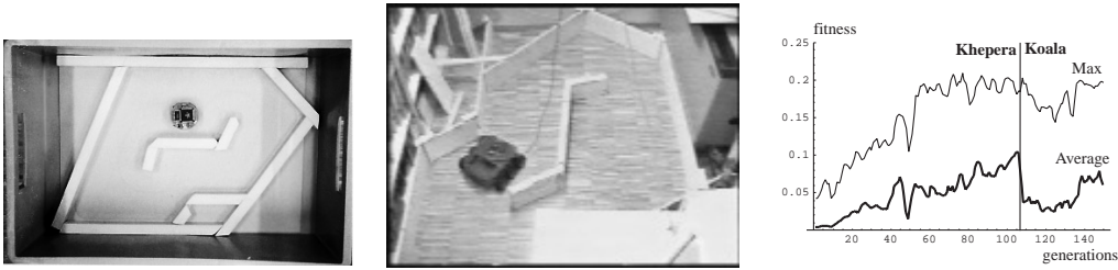
Figure 4: Incremental evolution across different robots. An initial population is evolved for navigation abilities on the miniature mobile robot Khepera (left). After 100 generations the population is transferred on the larger Koala robot and incrementally evolved using the same fitness function (center). The population quickly re-adapts to the new morphology and sensor characteristics, as shown by the fitness data (right) [10].
