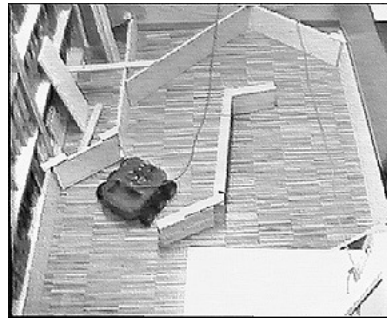
Figure 4: Incremental evolution across platforms. Initially a neural control system has been evolved using a miniature mobile robot Khepera. After 100 generations, the last population has been transferred on the much larger and more powerful Koala robot shown in the figure and evolution has been resumed. The population takes 20 generations to readapt to the new sensors, motors, and geometry of the larger robot.
