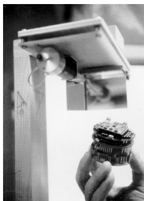
Figure 2. A close view of the robot with the "helmet" for capturing laser signals and the laser device on the background.
