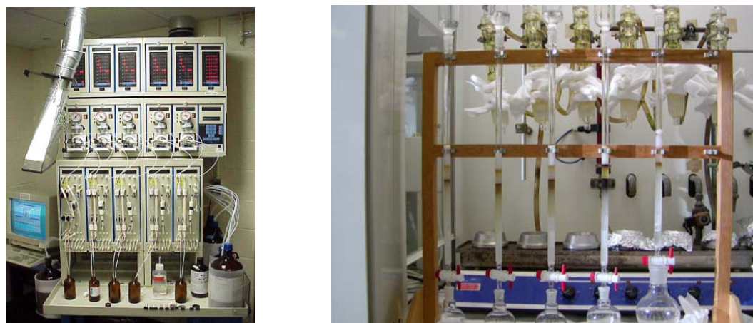
Fig. 3.4 The FMS system (in the left) and manual column (in the right)
