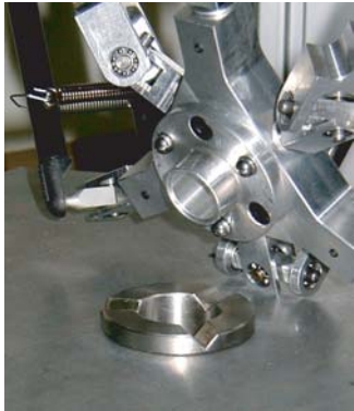
Figure 11: The Parking-System used for Initialization of the Robot. This systems consists of three spheres placed on the end-effector and three v-shaped grooves on the workbench. When applying a light vertical force (own gravitational force) on the end-effector when the spheres are roughly engaged into the grooves the whole system will center itself and guarantee a perfect positioning for initializing the robot.
