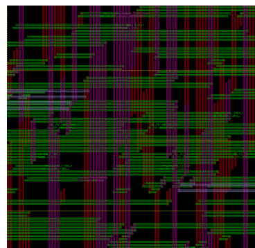
Figure 5 A closer view to the layout of the RC4 block that is routed fully differential wiring. The cell layouts are omitted for better visibility of the differential routing.
