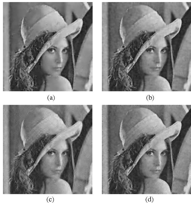
Fig. 9. Comparison of different smoothing methods. (a) Final multiscale B-spline-weighted Savitzky–Golay output (SNR = 27.30 dB). (b) Final multiscale nonweighted Savitzky–Golay output (SNR = 26.42 dB). (c) Wavelet thresholded image (SNR = 24.89 dB). (d) Wiener filtered image (SNR = 25.96 dB).
