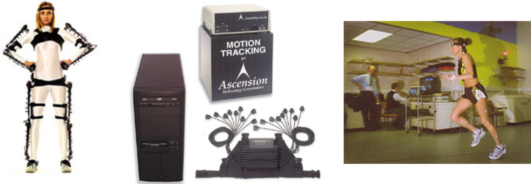
Figure 2.4: Motion capture systems. From left to right: Mechanical system ([Gypsy 4 ® , 2005]), Magnetic system ([MotionStar Wireless 2 ® , 2005]), Optical system ([Vicon Motion System ® , 2005]).
