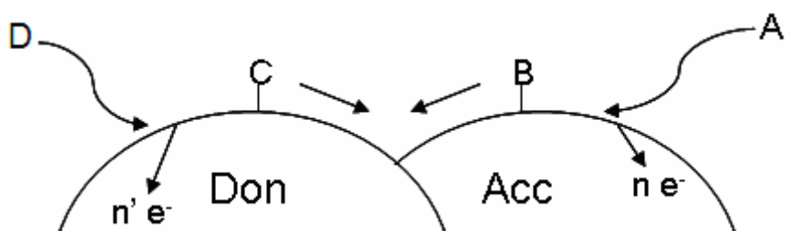
Figure 9.3: Schematic view of an electrochemical reaction at a surface composed of a donor (Don) and an acceptor (Acc) phase.
