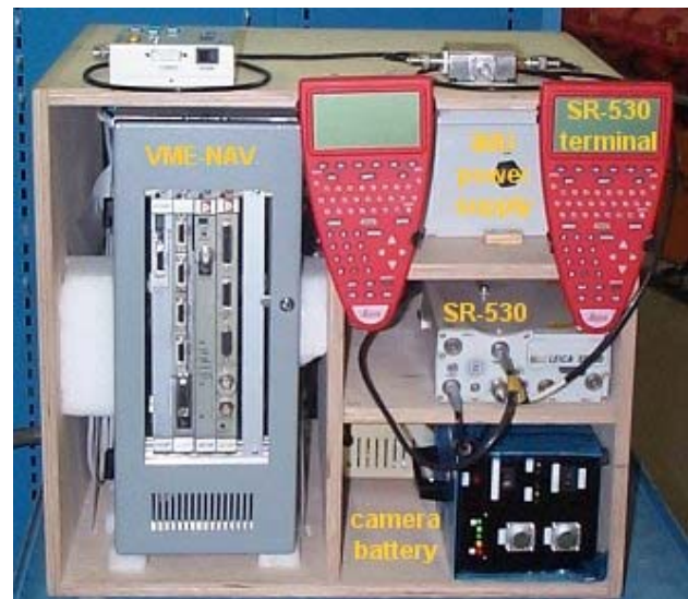
Figure 2. The sensor supporting electronic that is quickly installable.
