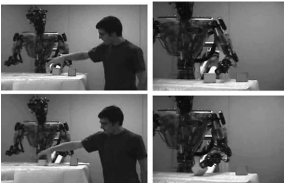
Fig. 2. Left: observation phase—the demonstrator moves each box from left to right. Right: ATR DB robot imitates the invariant of the demonstration, a motion of any block along the x -axis.
