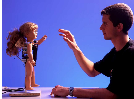
Figure 2: A PocketPC mounted with a FlyCam Camera tracks the motion of the user and sends commands to the microcontrollers and servos of Robota, so that it can imitate the motion of the head and arms of a user.
