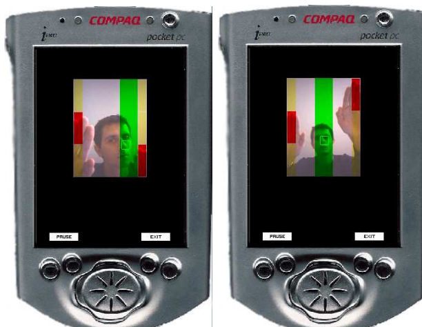
Fig. 2. Screenshot of the language acquisition application running on the iPAQ . The user has a visual feedback of his movements captured by the camera, with colored areas where the tracking take place.
