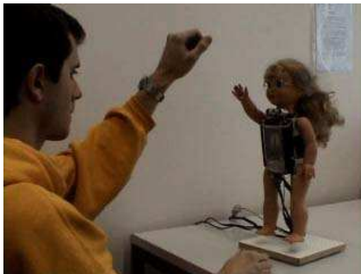
Fig. 4. Robota mirrors the motion of the user's arm. A PDA with a camera, mounted on Robota 's belly, tracks the motion of the user's arms and face continuously. A speech processing engine running on the PDA tracks the user's verbal input. The robot learn the meaning of the vocal utterance (e.g. "This is your arm") by associating the user's verbal input with its arms and face motion.
