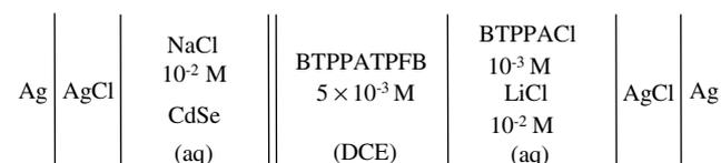
Fig. 1. The composition of the electrochemical cell.
