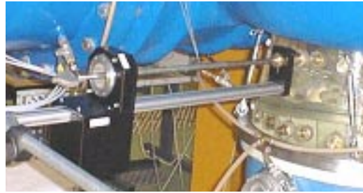
Figure 9 Five holes pressure probe mounted on the 2 axes remote traversing system
