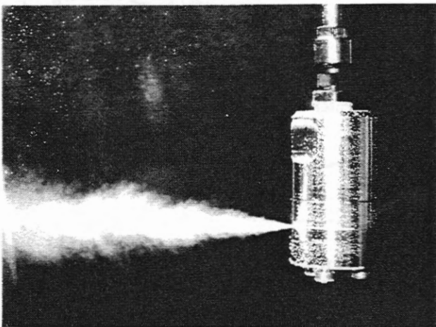
FIG. 16 INJECTION OF MICRO-BUBBLES.
