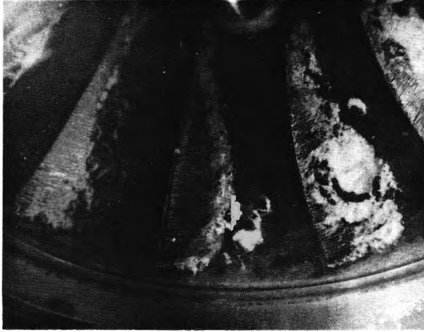
Fig. 1. Travelling cavitation vortices downstream the leading edge cavitation of a pump-turbine runner model in pump operation.
