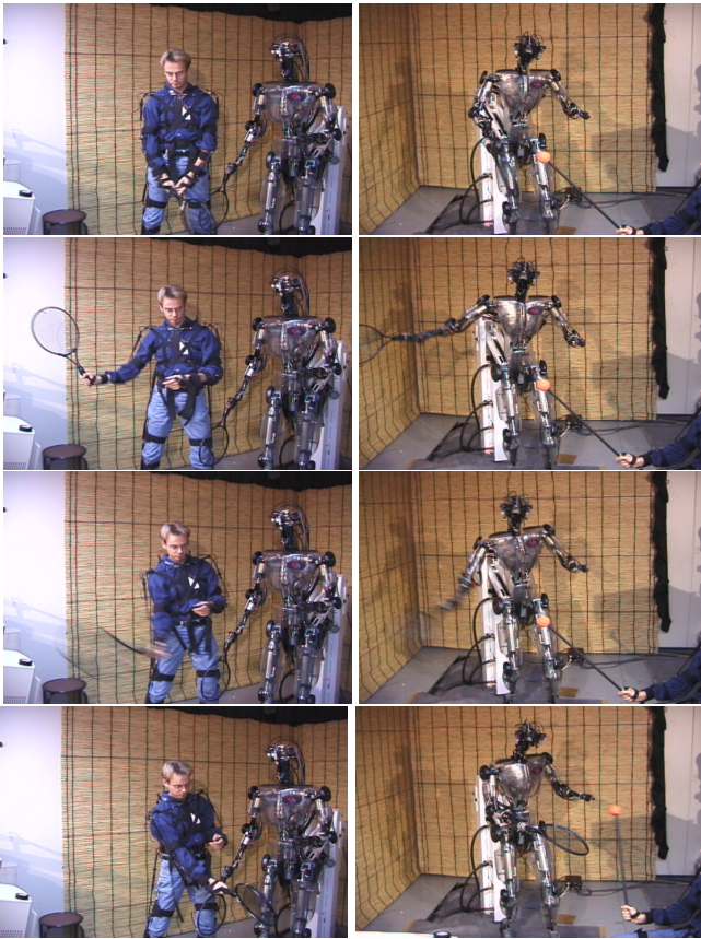
Figure 9: Humanoid robot learning a forehand swing from a human demonstration.
