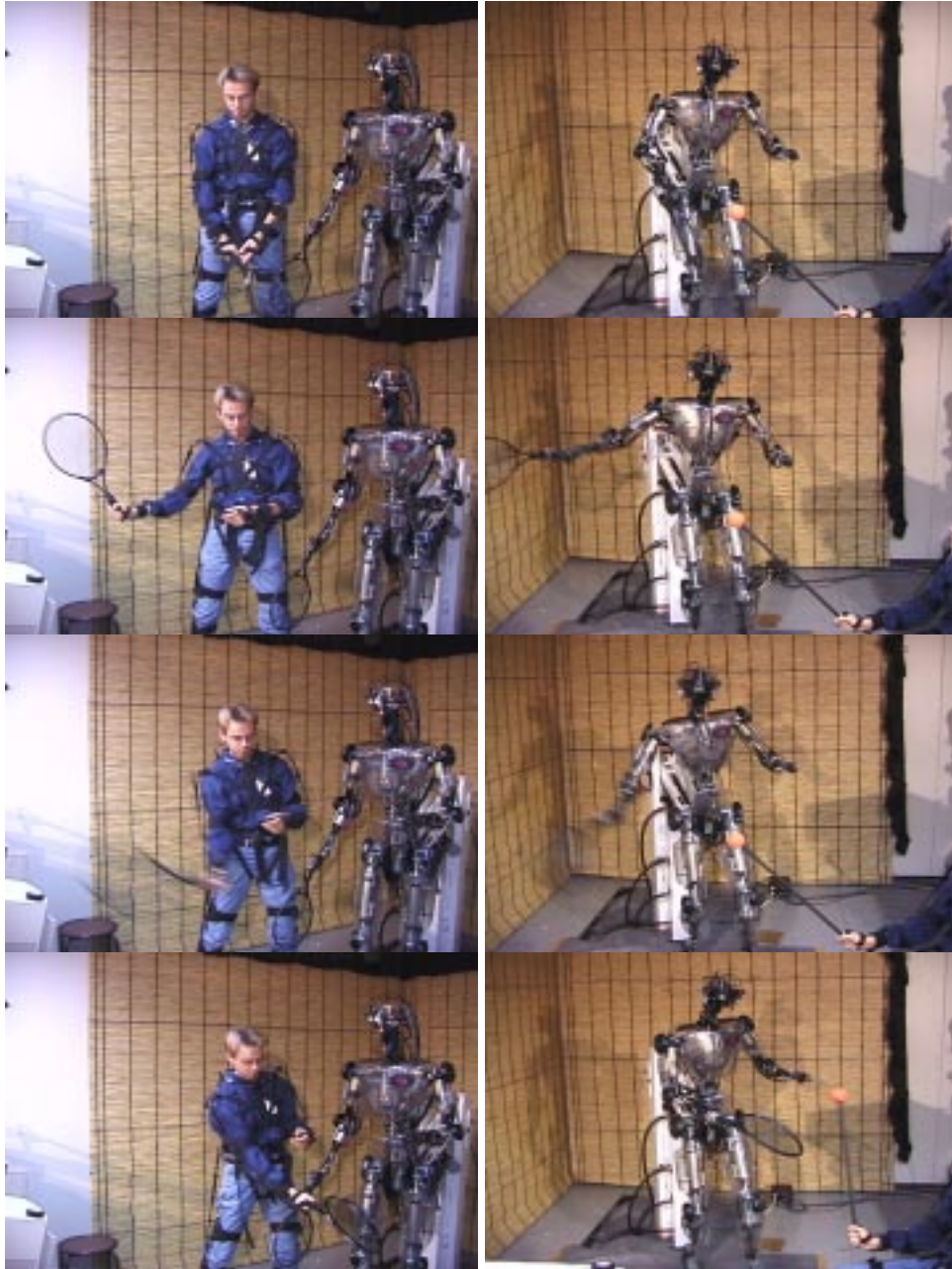
Figure 4: Imitation learning of a tennis forehand. The left column shows the teacher's movement, the right column the robot's movement towards a visually observed tennis ball.
