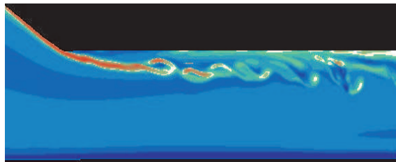
Figure 2.4: Vorticity in the downfield zone of a bypass: 2D details at the incoming branch (from a numerical simulation carried out by Fischer, Lee, Loth; University of Illinois and Argonne National Laboratories by permission).
