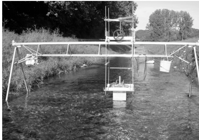
Figure 3 – Deployable 3D ADVP placed in the river Venoge. The ADVP transducers are installed inside the grey housing
