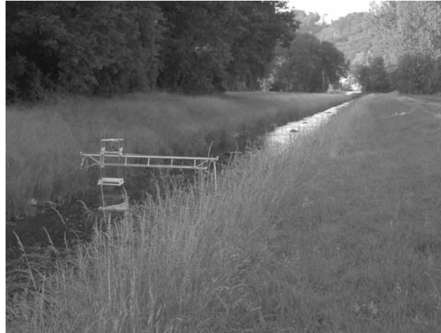
Figure 1. View of the study reach and of the deployable support structure for the ADVP field measurements.
