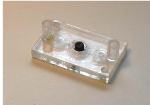
Figure 4 : Electromagnetic membrane micropump with 2 check-valves (dimensions: 36 x 22 x 5 mm, 7 layers).
