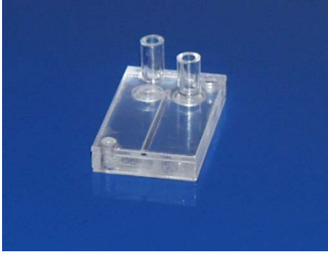
Figure 1 : Ferrofluid micropump (dimensions: 36 x 22 x 5 mm, 8 layers).
