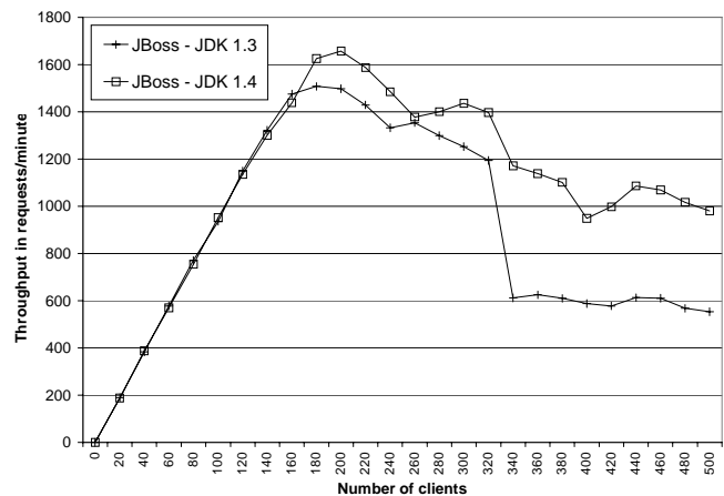
Figure 26. Session façade implementation throughput in interactions per minute as a function of number of clients for the bidding mix using JBoss 2.4.4 using JDK 1.3 and 1.4.
