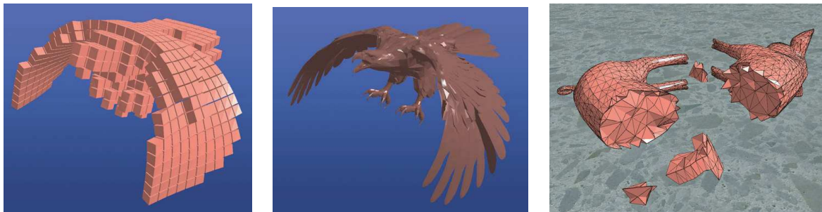
Figure 3.21: Deformable eagle FEM cube mesh (a) and surface mesh (b). A fractured pig model (c). (adapted from [Müller et al., 2004]).
