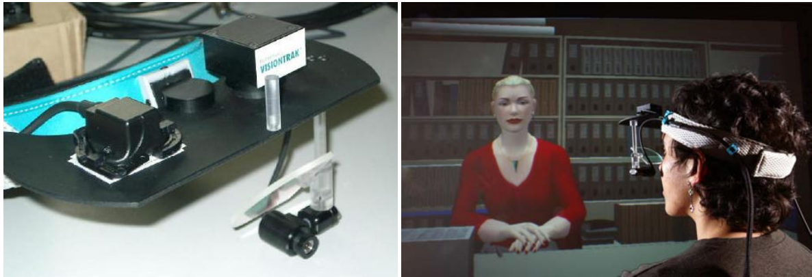
(a) VisionTrack device with mounted 6 DOF sensor (b) User wearing VisionTrack and facing the back projection screen
