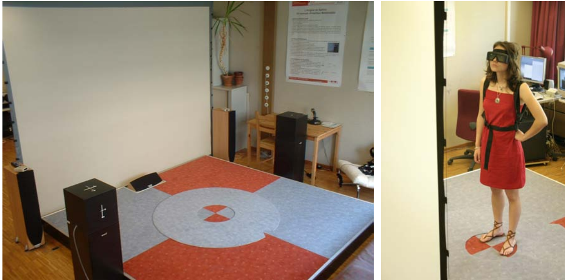
Figure 3.3: Large back-projection screen setup; the user wears CrystalEyes glasses and a MotionStar head tracker.
